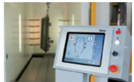
The control and command of height, width and depth detection are easily executed via monitor with touch-screen function and large display. Clear symbols offer a simple and intuitive operation. The coating programs and production data are stored on CompactFlash cards and can be recalled at any time.
