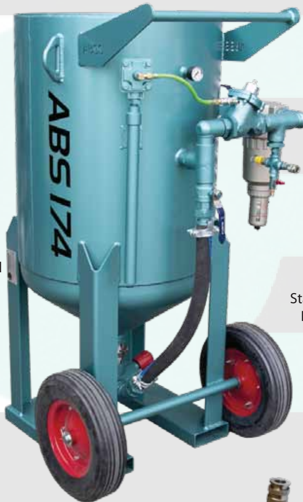
SMC 1-1/2" BSP Quality Filter on Solid 1-1/4" Piping
