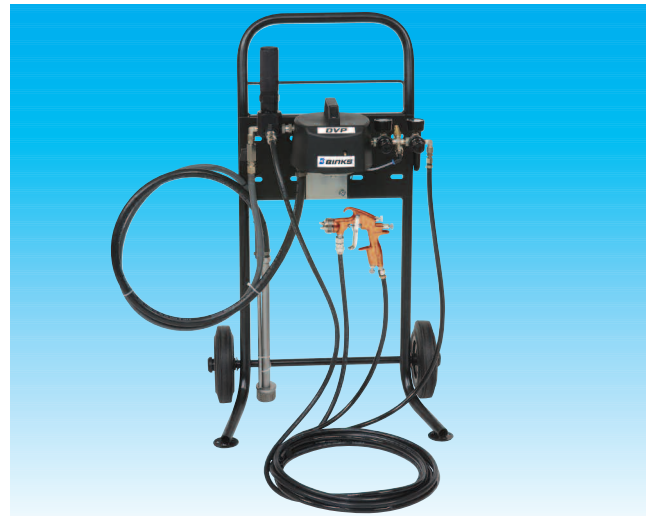
DVPAN-C-ADV: Cart-mounted waterborne pump, fluid filter/bypass assembly, twin air regulators, 7.5m air and fluid hoses, flexible suction wand and Advance Trans-Tech® Spray Gun*
