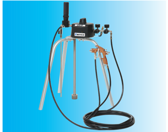
DVPAN-T-ADV: Tripod-mounted waterborne pump, fluid filter/ bypass assembly, twin air regulators, 7.5m air and fluid hoses, stainless steel pick up tube and filter and Advance Trans-Tech® Spray Gun*
